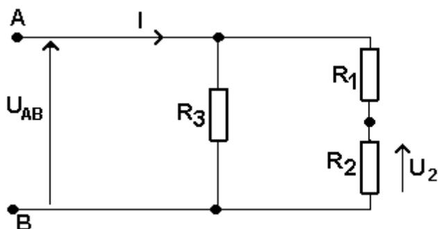
$R_1 = R_2 = R_3 = 1k\Omega; U_{AB} = 10V$
