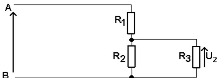
$R_1 = R_2 = R_3 = 1k\Omega; U_{AB} = 10V$
