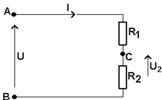
$U = 12V; R_1 = 1k\Omega; R_2 = 500\Omega$
