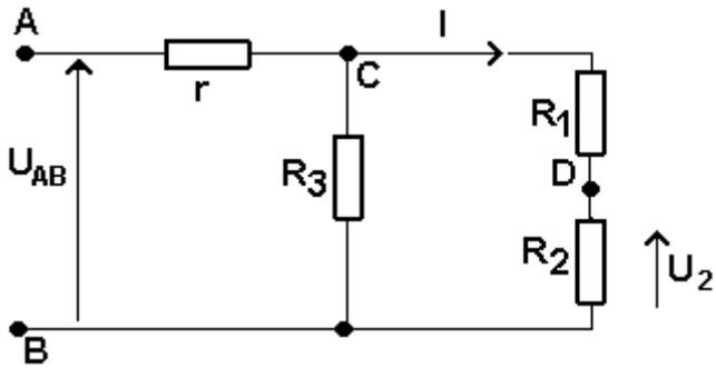
$r = 50\Omega; R_1 = R_2 = R_3 = 100\Omega; U_{AB} = 10V$
